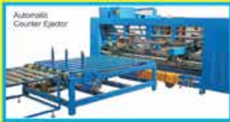
AS 016 - Semi Auto Stitcher AS 016A- Semi Auto Stitcher with Servo Drive
