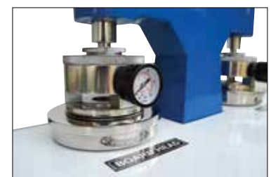
Manual Clamping System with Clamp Pressure Indicators
