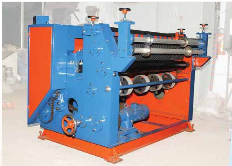
Sheet Cutter : Servo Motor Cut to length model available
