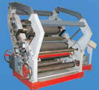
HD-180 Dual Flute Single Facer Speed : 70 M/ Min
