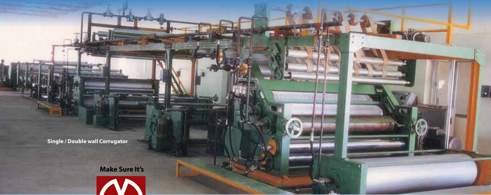
H-350 Fingerless Single Facer Speed : 150 M/ Min
