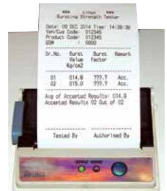
Printed Test Results by In-Built Thermal Printer
